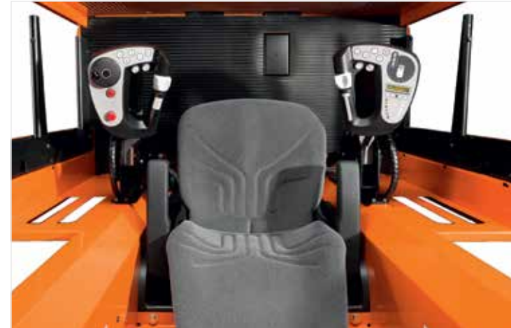
Split control panel lets the operator reach the pallet easily for order picking
